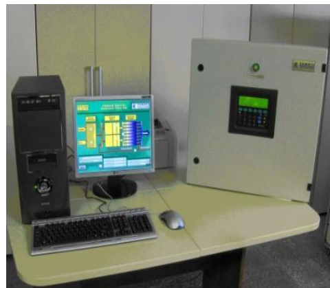
Wastewater Treatment Plant Monitoring and Control
