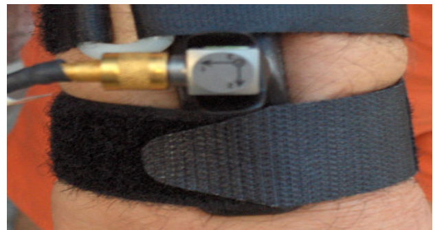
Fig. 4. Triaxial Accelerometer attached to the forearm human operator
