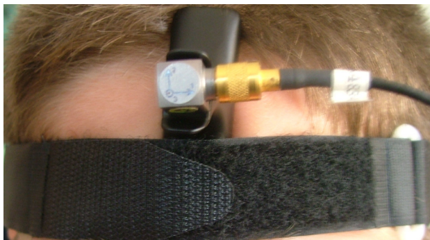
Fig. 3. Vibration measurements on the operator head
