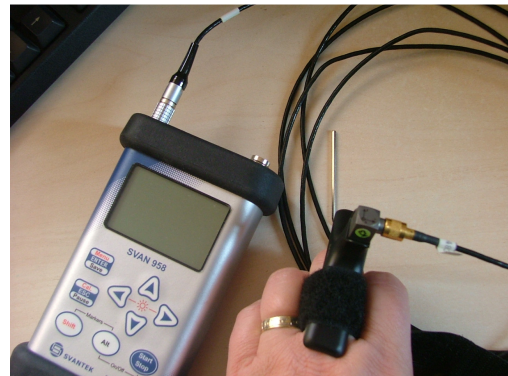
Fig. 2. Vibro-meter and the uni-directional accelerometer
