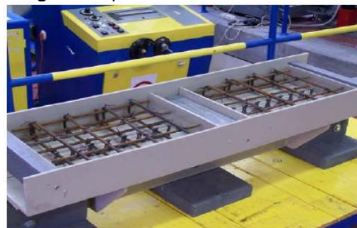
Fig. 4. Model of sheet types with indented cut forms
