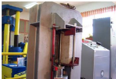
Fig. 5. Single push out test for sheet type with indented cut forms
