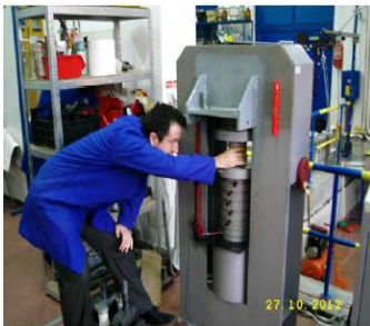
Fig. 1. Compression test on concrete cylinder
