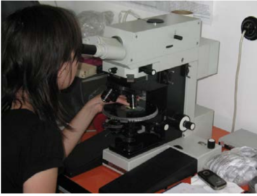
Fig. 1 Microscope Pol-U JENAPOL Determinations in reflected and transmitted light for the rocks and metallic minerals
