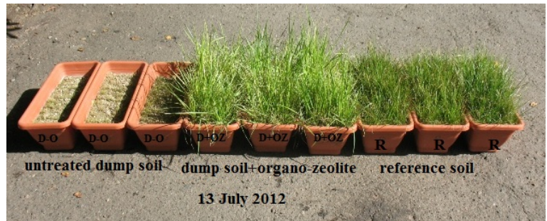
Fig. 4 Growth of the Lolium perenne specie on the "soil" from mining waste treated with the natural amendment (In collaboration with Department of Ecology and Environmental Education, Matej Bel University, Banská Bystrica Slovakia)
